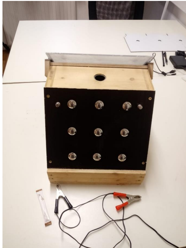
Figure 2. Back part of the apparatus, on the experimenter's side, where the nine buttons corresponding to the nine lights are placed. The hole where the rewards are placed is visible, as are the cables used to charge the battery of the apparatus. © P.Anibal
