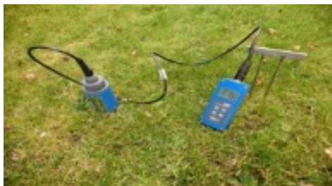
Fig. 6: Soil Moisture Probe
