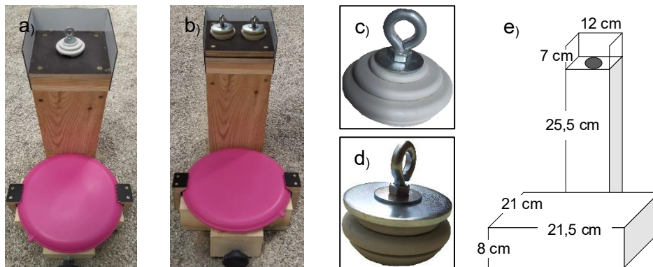
Figure 1: a) the apparatus used during training 1A, training 1B and test 1 with one grey plastic lid (basic lid) closing the top compartment and a pad mounted on the platform (pink). b) the apparatus used during test 2 with two grey plastic lids (metal washer lid) closing the top compartments and a pad mounted on the platform. c) basic lid with the ring bolt screw at the top and the plastic part at the bottom. d) metal washer lid with the ring bolt screw at the top, followed by the metal washer and the plastic part at the bottom. e) sketch with measurements of the apparatus.
