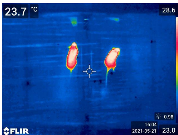
Figure 5: FLIR temperature picture showing 2 mice which can be measured simultaneously in 2 separate cages.
