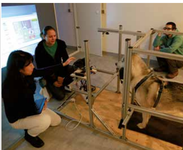
The eye tracker tracks the eye movements of dogs when watching pictures.
