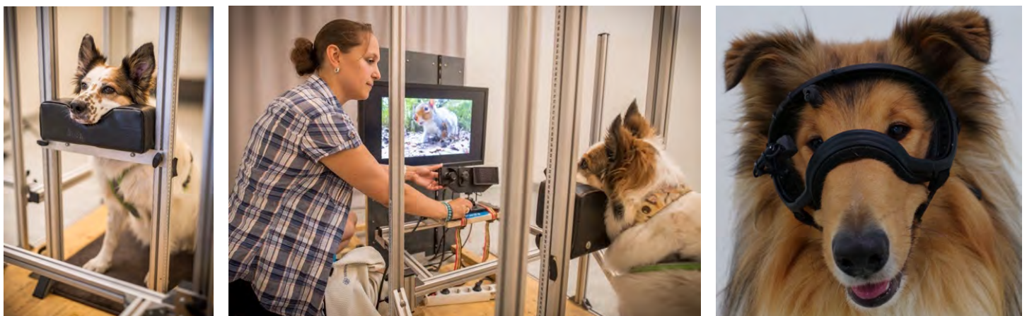
Figure 4. Figure 3. Snapshots of dogs in the Clever Dog Lab Vienna. Left and center: stationary eye tracking with the aid of a chin rest. Right: a dog with eye-tracking goggles.
