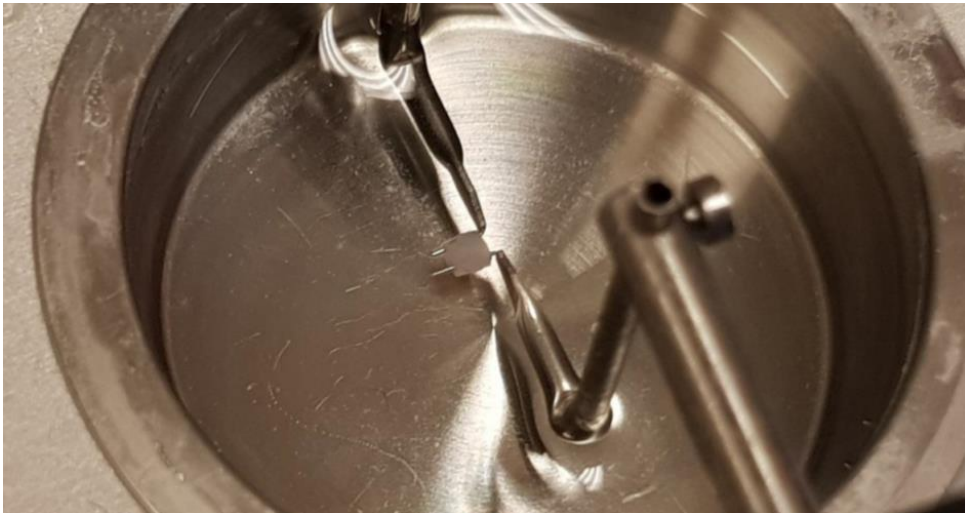
Figure 7: Organ bath chamber of the myograph with 200 \mu m hooks installed, after mounting an aortic segment (Photo: Christopher Dostal)
