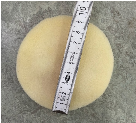
Figure 5: Circular foam piece (9.5 cm diameter, 1.5 cm height)
