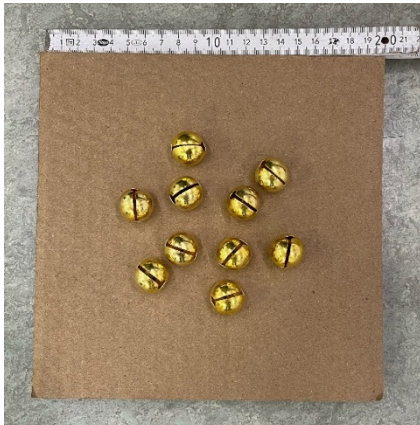
Figure 1: 20x20 cm lid with 10 bells (silent or noisy) attached
