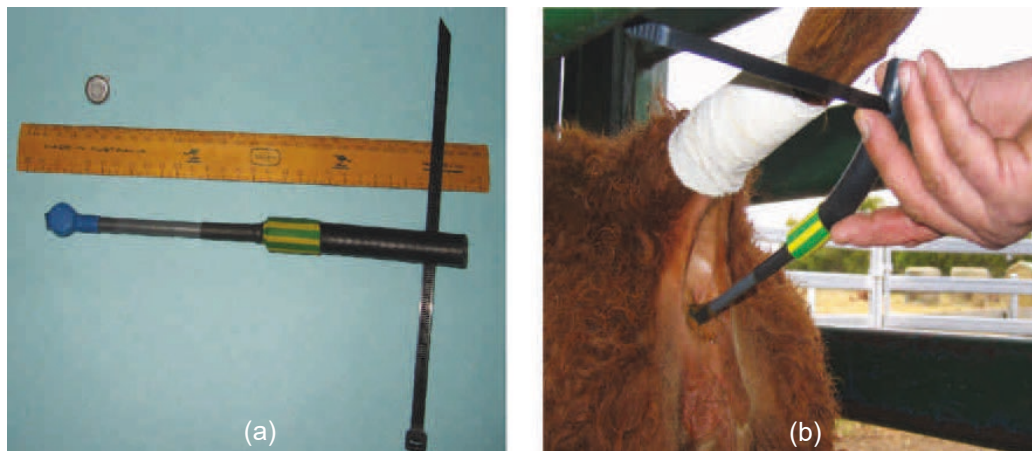
Figure 2. Device to monitor rectal temperature automatically in cattle. (a) Rectal probe with temperature logger and (b) attachment of the rectal logger probe to the tail (Lea et al., 2008).
