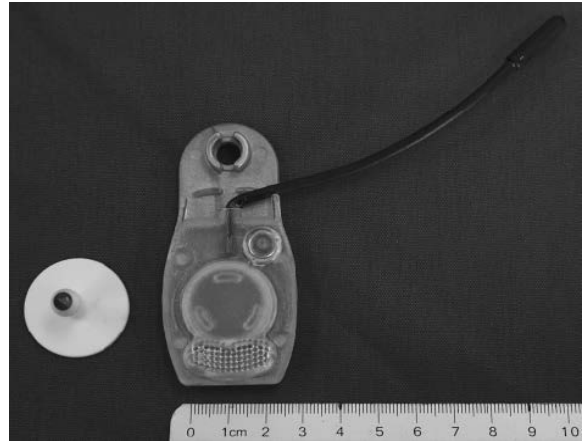
Figure 5. Fever Tag® temperature sensing ear tag (McCorkell et al., 2014).
