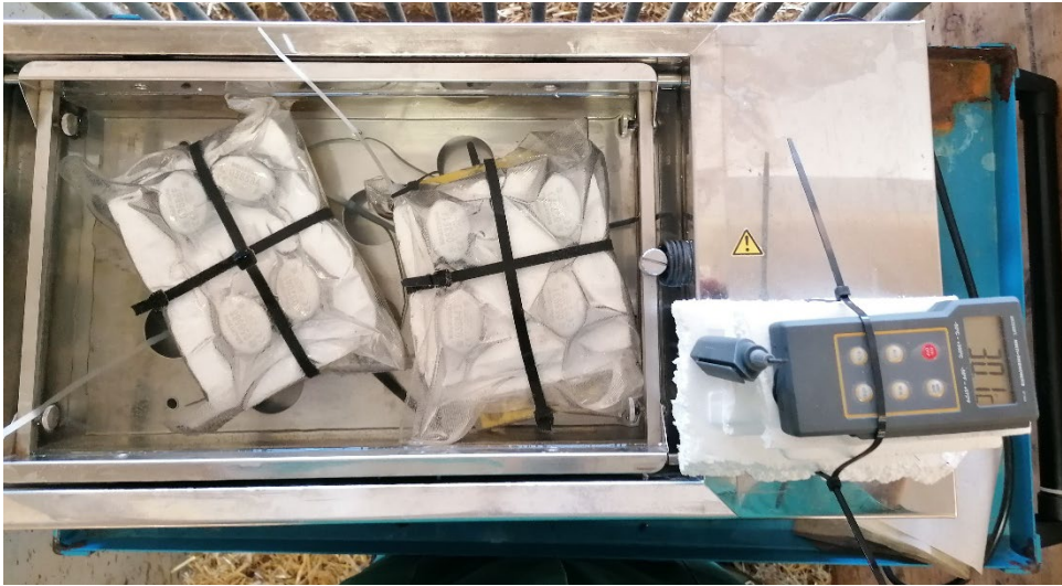
Figure 6. Ear tags positioned in a water bath, attached to Styrofoam plates and vacuum sealed.
