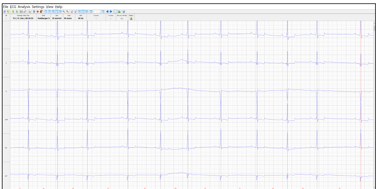
Fig. 3. Televet software surface. ECG recording with six leads (Einthoven leads I, II, III and Goldberger leads aVL, aVR, aVF). The R-waves are marked with vertical black dotted and red lines.
