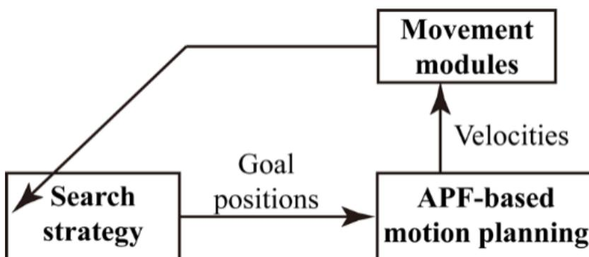
Figure 4: Control architecture for robot-based OF.
