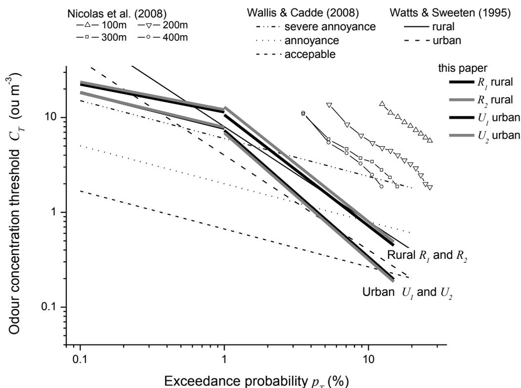
Figure 1: Relationship between exceedance probability  $p_T$  and odour concentration threshold  $C_T$  to define similar protection levels. The empirically derived functions are compared with the functions of Watts and Sweeten (1995) and Wallis and Cadde (2008). Additionally, empirical data are added for a pig farm (Nicolas et al., 2008a) (from Sommer-Quabach et al. (2014))
