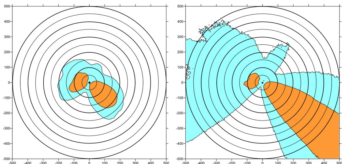
*Figure 2: Direction-dependent separation distances [m] with (left) AODM, peak-to-mean ratios from Fig.1, and (right) LASAT, factor 4, for 1 ou<sub>E</sub>/m<sup>3</sup> and 3 % (blue) and 8 % (orange) exceedence probability for Kittsee.*
