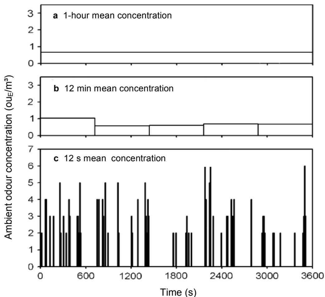
Figure 2: Time course of the odour concentration ( $ou_E / m^3$ ) for three time intervals. (a) one-hour mean value (e.g. output of a dispersion model), (b) 12-min and (c) 12-s mean odour concentrations observed at a single receptor point during a field study. The 12-s mean values were recorded and subsequently used to calculate 12-min and one-hour mean concentrations (source: Schaubberger et al. (2012c), modified from Nicell (2009)).
