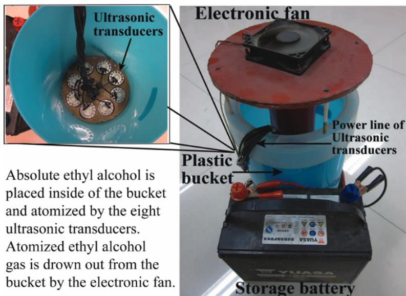
Figure 2: The schematic of the electronic nose
