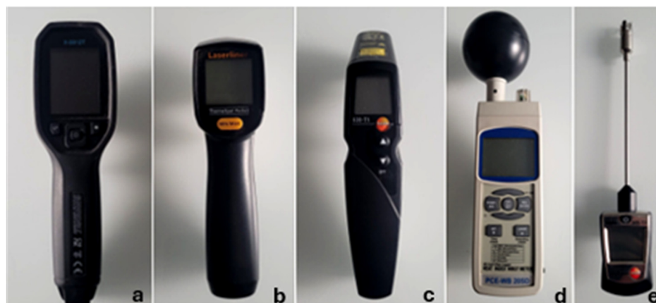
Figure 7. The measurement devices used in the present study. (a) FLIR TG165-X MSX (FLIR, Täby, Sweden) Thermal Camera for infrared thermography, (b) Laserliner ThermoSpotPocket thermometer (Umabrex, Arnsberg, Germany), (used for infrared thermography), (c) Testo: 830-T1 thermometer (Testo Austria, Vienna, Austria) used for infrared thermography, (d) heat index WBGT metre PCE-WB 20 SD (PCE, Meschede, Germany) used for meteorological measurements, and (e) surface thermometer Testo 905-T2 (Testo Austria, Vienna, Austria) used for measuring the temperature of the mouthpiece. Photo by the authors.
