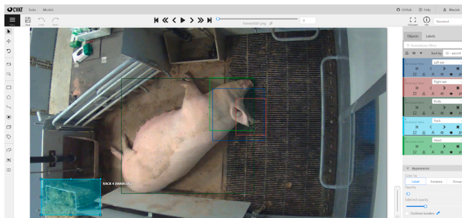
Fig. 2. Labelling of a video frame in CVAT. Objects labelled: left ear, right ear, head, body and the hay rack. A hay rack is highlighted in the figure as it is selected by the mouse pointer. Ear tag with an accelerometer is placed on the left ear of the sow.
