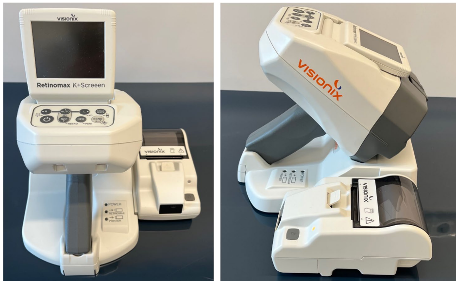
FIGURE 1 | The handheld autorefractometer Retinomax K+ Screen (Visionix), shown in front view (left) and side view (right), mounted on its charging and printing station.
