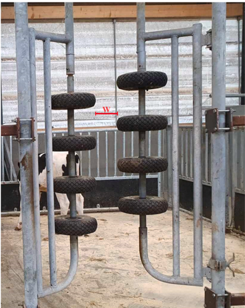
Fig. 3. A photo of one of the push gates. The perceived width (W) between the two parts of the gate was 11 cm when fully closed, 52 cm when half-way open, and 67 cm when fully open.
