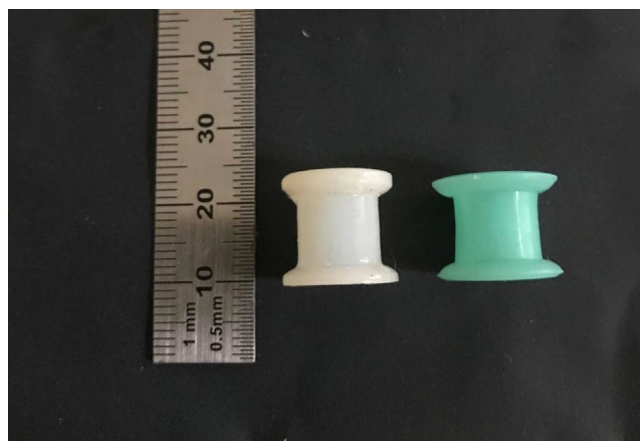
FIGURE 6 Comparative image of the 3D-printed silicone stent on the left and the commercially available stent on the right. Note the 1 mm increased length and rounded flanges of the 3D printed device.
