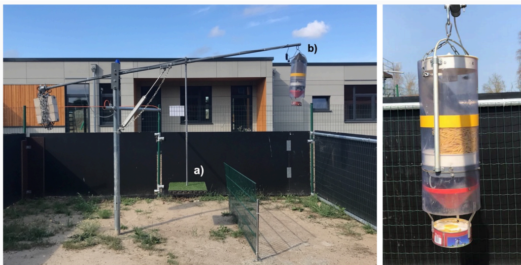
Figure 1. Left image: the test arena with the Fake Apple Tree apparatus on which the platform (a) and dispenser (b) were attached. Right image: the dispenser, containing raw pasta, attached to the pivoting arm.
