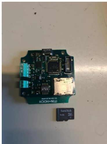
Figures 2 and 3: inside of the RumiWatch (RumiWatch System, ITIN + Hoch GmbH, Liestal, Switzerland), showing the battery and the data logger with the SD card (pictures by Raul Rivera Chacon).
