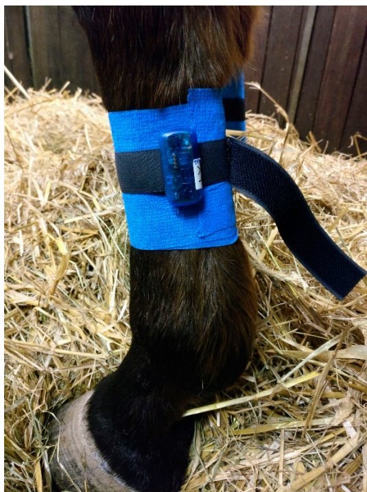
Figure 1. The method of attaching the accelerometers (MSR145, sampling rate: 1 Hz, and measuring range: \pm 15 g) to the equine extremity laterally in the mid-region of the metacarpal and metatarsal bone with a Velcro fastener and one layer of elastic band.
