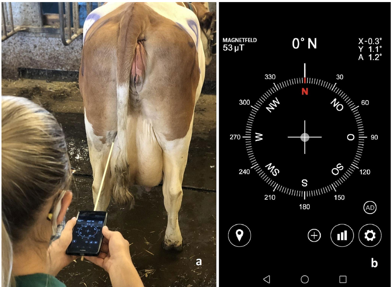
Fig. 2 Measuring longitude and latitude using the compass app (COMP) on the smartphone. A wooden stick was attached to the back of the smartphone to support the measurement process (a). Screenshot
