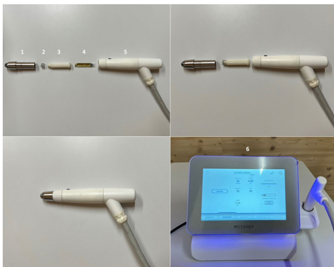
1) applicator tip, 2) TDA pen, 3) cartridge case, 4) cartridge, 5) applicator body, 6) DERMADROP device
