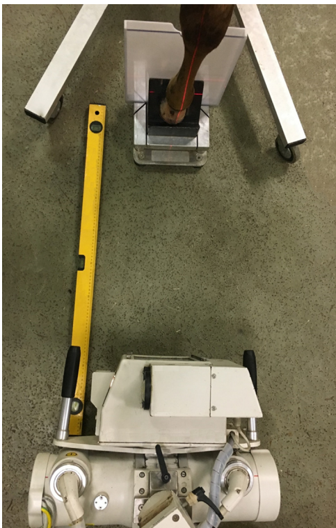
Fig. 5. Experimental setting for image series of a cadaver limb. The detector, embedded in the cover box, is capable to store all the image of one series. Consequently, there was no need for any changes to the condition of admission. For a new image exclusively the mAs-settings had to be changed at the control panel.
