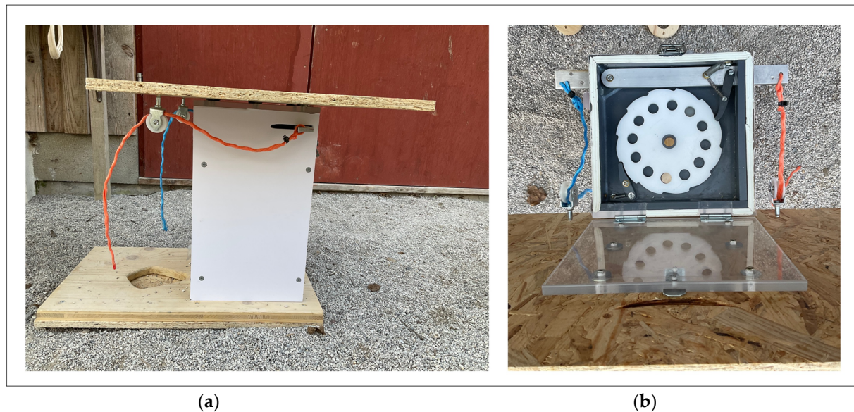
Figure 6. Photographs of the experimental box. (a) Side view of the box showing the functional (red) string attached to a lever and threaded through a pulley. When this string is pulled, a small piece of peanut is released into the reward tray at the bottom. (b) Top view of box with open lid. By pulling the string, a lever moves and turns the hopper to release a peanut. Only the red string on the right is functional. The blue string is attached to a dummy lever and is non-functional.
