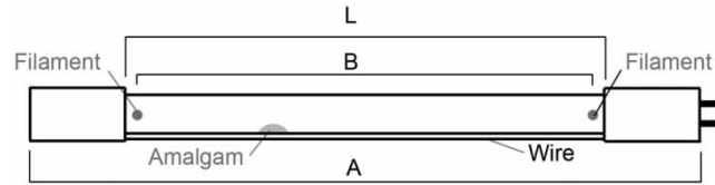
Figure 3 | Schematics of an amalgam-LP-high-output lamp, whereas A denotes the total length of the lamp, L the length of the uncovered glass bulb and B the distance between the spiral-wound filaments. In some lamps, the ends of the glass bulb and in some lamps also the filaments are hidden by the socket. In the last case: B > L .
