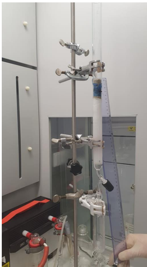
Figure 3. Experimental setup for VLC. The loaded column was placed on a dripping funnel and connected to a vacuum pump. With the closed stop of the dripping funnel, each 20 mL of eluent mixture was placed on top of the column and elution was slowly initiated by vacuum. After most of the eluent has passed through the column and collected in the dripping funnel, the vacuum was disconnected and by opening the stop of the dripping funnel, the fraction was collected in 20 mL glass tubes. This was repeated 21 times.
