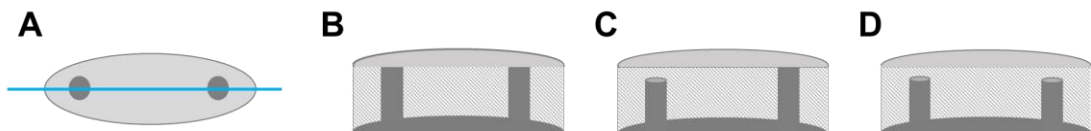
Figure 9: Pin variation. (A) Section through the main chamber for lateral view of B, C and D (B) Continuous design: both PDMS pins connected to the ceiling (C) Semi-continuous design: only one PDMS pin connected to the top layer (D) Non-continuous design: none of the PDMS pins reaches the ceiling
