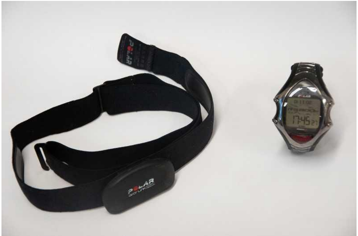
Fig. 3: Polar RS800CX heart rate monitor and accompanying electrode belt
