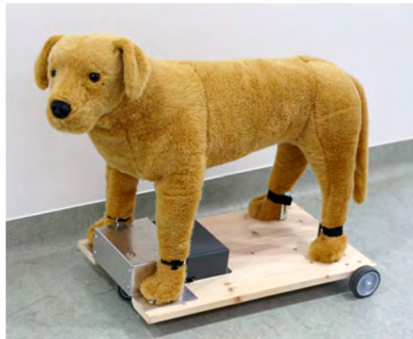
Figure 1. Fake dog mounted on board with wheels that could be moved via remote control.
