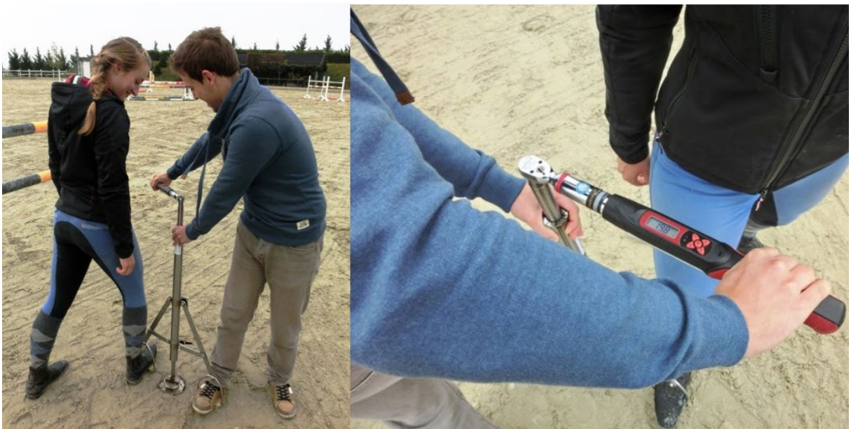
Figure 1: testing conducted on sand with the Vienna Grip Tester: the device is lowered on the ground, with the hoof application sitting flat on the surface. The person conducting the test and an assistant step into the steel stir-ups with their right foot, pressing them towards the ground to make contact with it. This assures that the applied force has the correct load of 700N on the gas spring, which is encompassed into the metal tube used as casing. The wrench shown in the right picture is then twisted 45 ° in order to take the measurement. The number on the display shows the grip measure in Nm.
